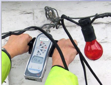
Pull test on anchorage points
