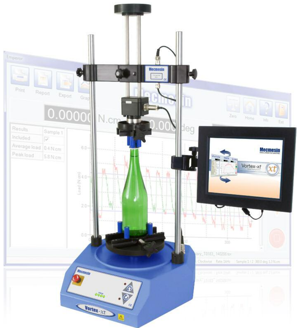
Opening test of beverage closure
