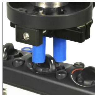
Automotive rotary switch torque test
