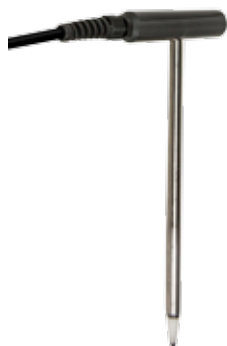
VPT Soil cell for soil conductivity
