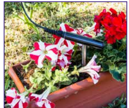
Measurement of conductivity in the soil
