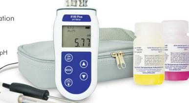
The pH readings are either manually or automatically temperature compensated over the range of 0 to 100 °C. To automatically compensate, it is necessary to utilise a thermistor temperature probe. Each unit incorporates an auto-power off facility that automatically turns the instrument off after ten minutes, maximising battery life.
