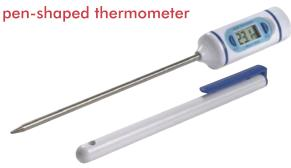
This pen-shaped thermometer measures temperature over the range of -49.9 to 149.9 °C, features a  $\emptyset 3.5 \times 120$  mm stainless steel penetration probe and incorporates a °C/°F switch and display hold feature. Supplied with a probe cover that includes a pocket clip.
