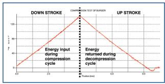
The energy put into the sample is absorbed, stored or returned. We measure this response and also present it in graphical form to aid in understanding and putting numbers to sensory characteristics. Instrumental results are almost always correlated to sensory panel judgements and sensory characteristics such as hardness, cohesiveness and stickiness can be calculated.
