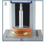
The texture analyzer's crosshead then travels to either a programmed distance or load, recording the force response of the sample to the deformation imposed.
