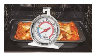
This stainless steel oven thermometer features a clear  $\varnothing 55$  mm dial with colour-coded zones. The green marker indicates the minimum temperature that commercial hot food display units should be kept at. The oven thermometer indicates temperature over the range of 0 to 300 °C in 10 °C divisions. The case measures  $43 \times 66 \times 80$  mm.
