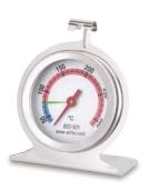
This stainless steel oven thermometer features a clear  $\varnothing 50$  mm dial with colour-coded zones. The green marker indicates the minimum temperature that commercial heated display units should be kept at. The oven thermometer indicates temperature over the range of 50 to 300 °C in 10 °C divisions. The case measures 40 x 60 x 70 mm.
