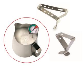
These stainless steel probe holders clip on the top of a jug, saucepan or similar to hold in place a temperature probe. Two models are available, one that will accept either a  $\emptyset 3$  or  $\emptyset 3.3$  mm probe stem and the other is designed to work in conjuction with a bi-metal thermometer and will accept a  $\emptyset 4$  mm probe stem. **Please note:** The probe should not touch the bottom or sides of the container.
