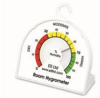
The general purpose hygrometer incorporates a 70 mm diameter dial with arrow indicator and colour-coded zones to display humidity levels e.g. dry, moderate and humid. The hygrometer indicates the level of humidity in 5 % divisions over the range of 0 to 90 %rh.
