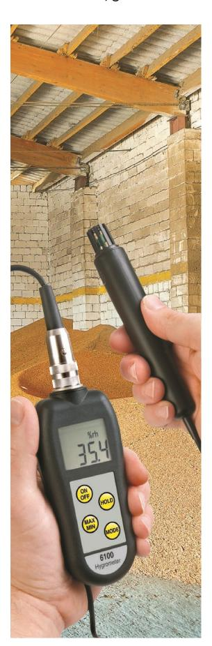
In many manufacturing processes the measurement of relative humidity (%rh) is important, as many products are sensitive to variations in humidity. Therefore humidity needs to be measured and controlled for the end products to be consistent in both quality and performance.
