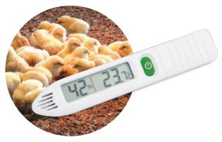
The pen-shaped hygrometer simultaneously displays both humidity and temperature over the range of 20 to 95 %rh and 0 to 49.9 °C.
