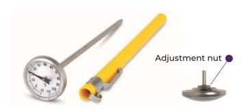
These pocket-sized  $\emptyset 25$  mm dial thermometers feature a magnified lens and a pointed  $\emptyset 4 \times 130$  mm stainless steel stem. Each dial is manufactured in three scales and is supplied with a FREE calibration spanner and probe cover complete with pocket clip.
