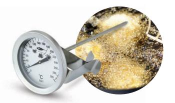
This frying thermometer incorporates a  $\emptyset$ 50 mm dial and a pointed, stainless steel  $\emptyset$ 4 x 150 mm probe and indicates temperature over the range of 0 to 300 °C in 10 °C divisions.
