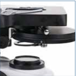
Zernike phase contrast condenser with filter holder
