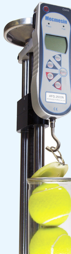
Packaging seal release force test
